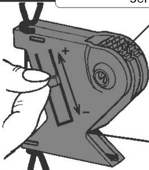
Adjust sensitivity with slider according to size and drag of lure being used.
