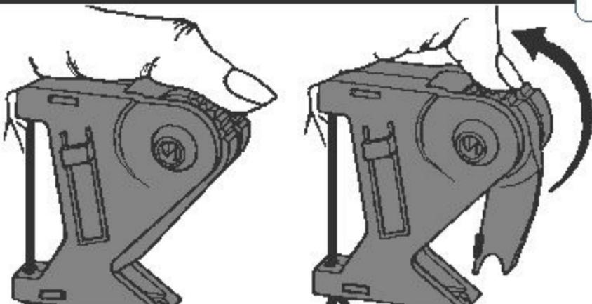
Open Release with thumb by pushing the slider to the upper position (See fig.) then turn holding plates towards direction shown by the arrow.
