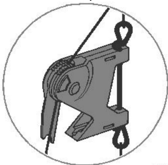
Fit the line through the lower notch of the lever
